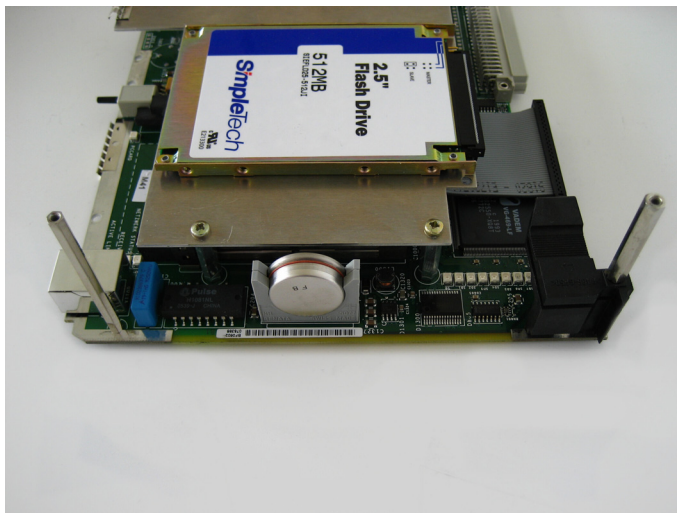
Figure 1-9 Battery on the CPU module
