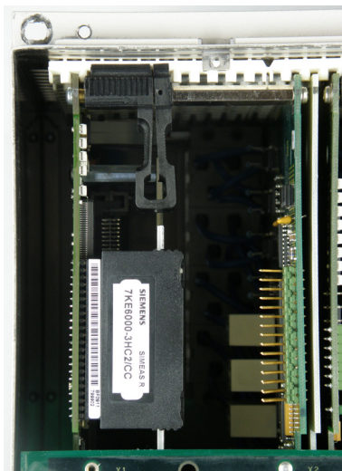
Figure 3-16 DOM Flash Memory on the CPU module
