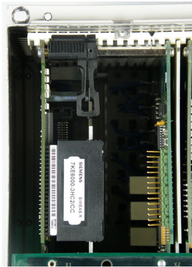
Figure 3-15 Installed DOM Flash Memory
