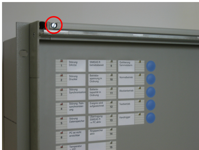
Figure 1-1 Removing the cover frame
