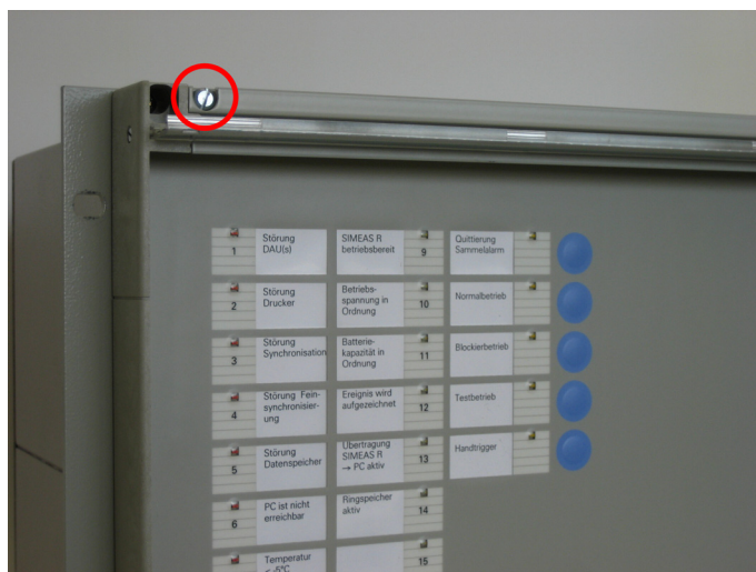
Figure 1-10 Removing the cover frame
