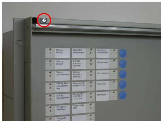
Figure 2-1 Removing the cover frame
